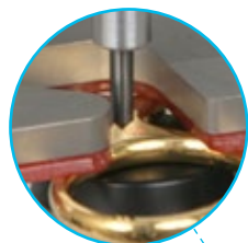
Marking machine Travel: 40 x 40 mm (1.6 x 1.6 in.)
