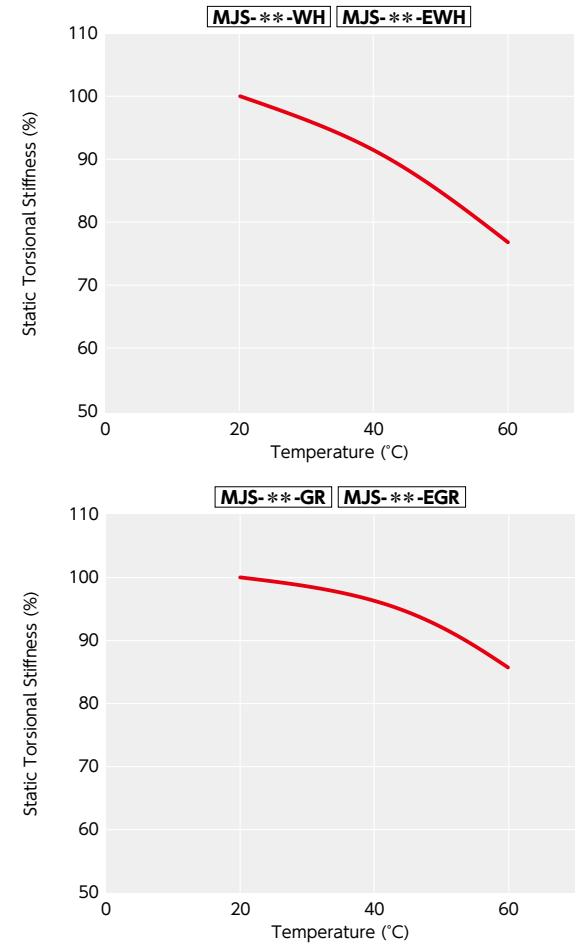
This is a value under the condition where the static torsional stiffness at 20°C is 100%.
