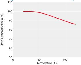
This is a value under the condition where the static torsional stiffness at 20℃ is 100%.
