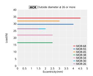
This is a value under the condition where the static torsional stiffness at  $20^{\circ}$  is 100%.
