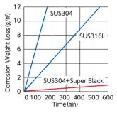
This graph compares corrosion weight loss of a test piece in 6% ferric chloride solution over time. After the same length of time, the corrosion weight loss of super black is much less than that
