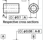
(reproduced) center of the outside circle must be within the circle concentric with datum circle A and of 0.1 in diameter.
