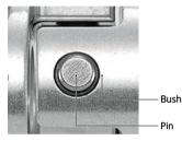
The high accuracy fitting of pin and bush allows the extremely small backlash. For the bush of **XUT** the polyimide resin with excellent abrasion-resistance is adopted. The backlash at the initial stage is maintained for a long period.
