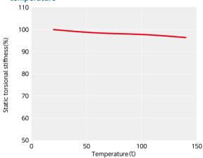
This is a value under the condition where the static torsional stiffness at  $20^{\circ}$  is 100%.
