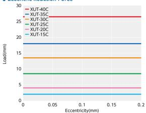
**XUT** has small eccentric reaction force and an extremely small shaft load generated by misalignment. This reduces the load to such components as shaft bearings.
