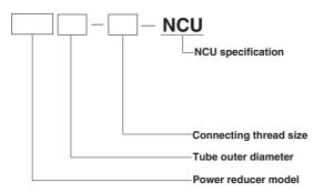
※ For the fitting models, the tube size, and thread combinations, see the table below. Columns showing the "←" symbol indicate that standard products can be used as the NCU specification. In these cases, place orders for the standard products.
