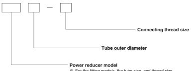
For the fitting models, the tube size, and thread size combinations, see the tables below.
