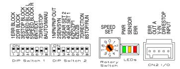
This configuration (factory set) is the standard set-up for any zone that is not specifically an infeed or discharge zone.
