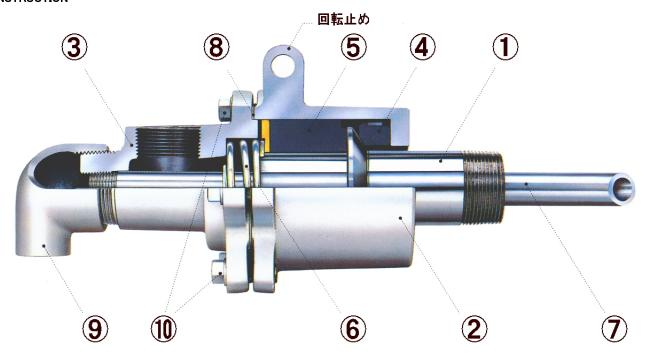
①ROTOR(CARBON STEEL) ②CASING(CASTING IRON) ③HEAD(CASTING IRON) ④SEAL RING(CARBON) ⑤CARBON BEARING ⑥SPRING (S.STEEL) ⑦INTERNAL PIPE ⑧GASKET ⑨ELBOW ⑩BOLT
