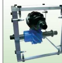
Installment : Nonparallel and nonintersecting gears
