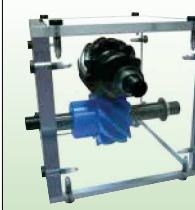
Installment : Nonparallel and nonintersecting gears
