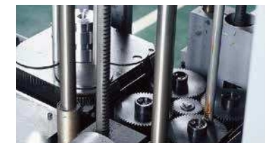
SRO Round Rack used as a work storage device (fluctuating table) of the auto loader.
