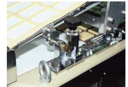
SW Worms and BG Worm Wheels used in adjusting a cloth feeding device
