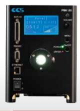
The supplied AC cord is for use with 100 to 120 VAC CCS recommends using the following with 200 to 240 VAC. Cable: GTCE-3 x 1.0 mm² (Kawasaki Electric Wire) Connector: KS-31AY (Kawasaki Electric Wire)
