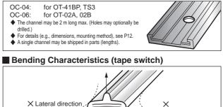
Perpendicular direction (up/down, permitting bending angle of R50 approx.)
