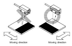
• Use the sensor in a way that the sensing surface of the sensor and the detection object surface are parallel. (The object must not be at a slant.)
