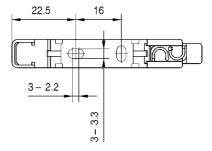
• When mounted on DIN rail
