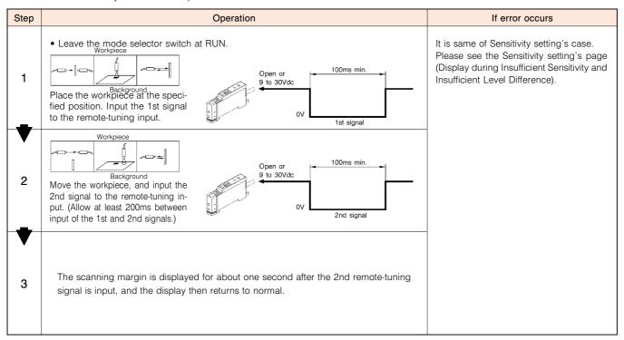
When the remote sensitivity is not set, either cut the pink lead (remote-tuning input lead) at the root of the cord, or connect it to + power supply terminal.
