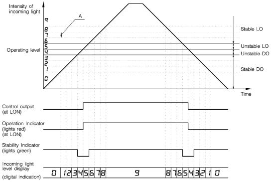
A: A double width of hysteresis, automatically set on sensitivity setting.
